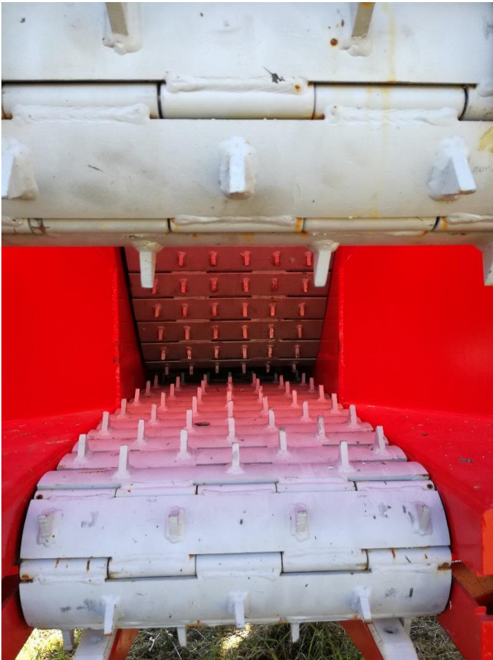
Figure 10 Wood (biomass) chipper loads small logs and branches. "Teeth" of this "jaw" chip and shred biomass into small pieces for further production.
